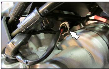
14 Unplug the stock wiring harness from the Crank Position Sensor.
