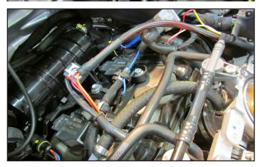
10 Unplug the stock wiring harness from each ignition coil.
