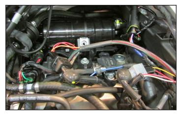
11 Plug the PC6 in-line of the stock wiring harness and each ignition coil.
