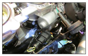
13 Plug the PC6 in-line of the stock wiring harness and TPS.
