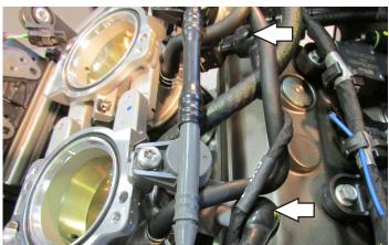
9 Plug the PC6 in-line of the stock wiring harness and each injector.
