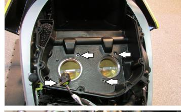
8 Unplug the stock wiring harness from each injector
