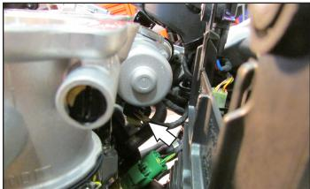
12 Unplug the stock wiring harness from the Throttle Position Sensor.
