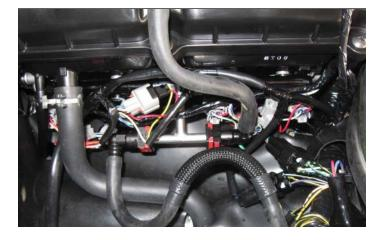
6 Attach the connectors from the PC6 to the stock wiring harness and each injector.
