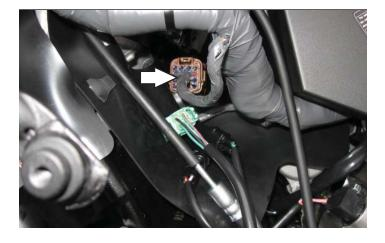
4 Unplug the stock wiring harness from the throttle bodies.
