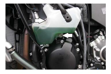
Remove the coolant reserve bottle by removing the two mounting bolts.
