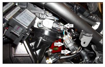
9 Unplug the stock wiring harness from each ignition coil.
