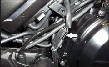
11 Locate the Crank Position Sensor connector. Unplug the CPS connector.
