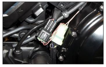
12 Connect the PC6 harness in-line of the CPS and stock wiring harness.
