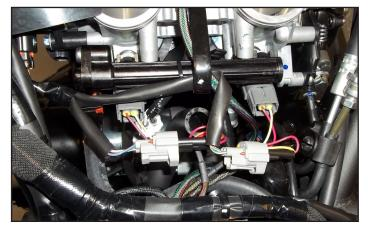
6 Locate the Throttle Position Sensor on the left side of the throttle bodies. Unplug the TPS.
