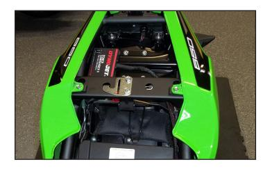
2 Lay the PC6 in the tail section and route the wiring harness down the left side of the frame, towards the throttle bodies.
