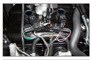
10 Connect the PC6 wiring harness in-line of the stock ignition coils and wiring harness.
