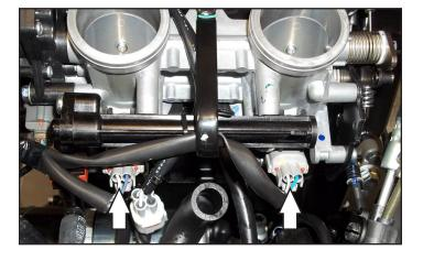
4 Unplug the stock wiring harness from the injectors.
