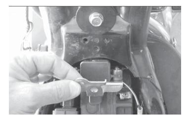
5 Unbolt and move the tip over switch out of the way.
