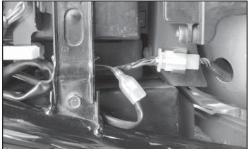
On Mean Streak models only, plug the PC6 ground wire with the male bullet connector into the stock auxiliary ground connector. The stock auxiliary ground connector is found next to the battery. It has a double female bullet connector and a BLACK/ YFLLOW wire.
