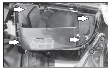
7 Route the PC6 wiring harness between the plastic tray and the left frame rail. Continue routing beneath the frame/lower fuel tank mount and towards the throttle body.
