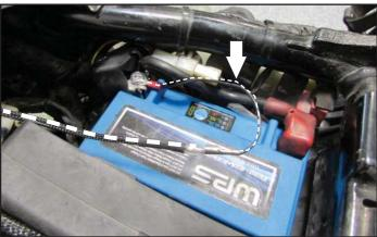
On VN1500 Drifter, Nomad, and Classic models, secure the supplied Ground Wire to the negative (-) terminal of the bike's battery. Plug the PC6 wiring harness into the Ground Wire.
