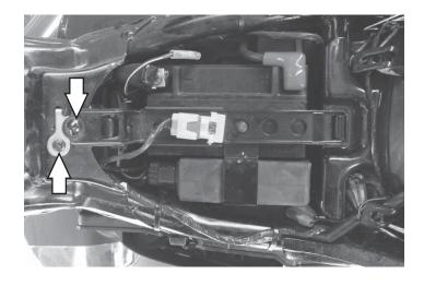
4 Remove the battery/ECU bracket.
