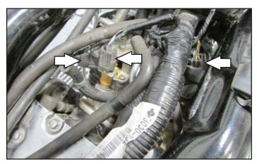
9 Use the supplied Posi-tap to attach the GREY wire of the PC6 wiring harness to the stock YELLOW/WHITE wire of the TPS connector. Plug the TPS connector back on to the TPS.
