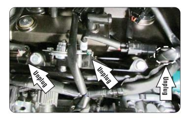
13 Unplug the stock wiring harness from all three of the bike's Fuel Injectors.
