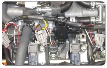
14 Plug the PC6 wiring harness in-line of each Fuel Injector and the stock wiring harness.
