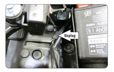
5 Locate and unplug the stock Crank Position Sensor connectors.
