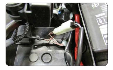
Plug the pair of PC6 connectors with BROWN colored wires in-line of the stock Crank Position Sensor connectors.
