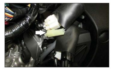
11 Plug the PC6 wiring harness in-line of the CPS and the stock wiring harness.
