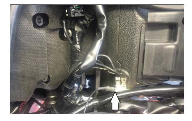
5 Attach the ground wire of the PC6 to the common ground location towards the rear of the engine.
