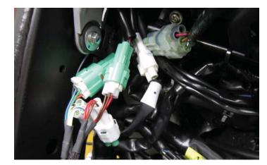
8 Unplug the wiring harness from the Throttle Position Sensor.
