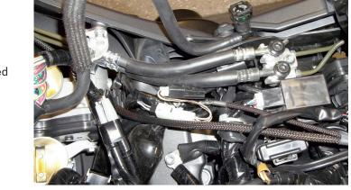
9 Unplug the stock Throttle Position Sensor (TPS) connector.
