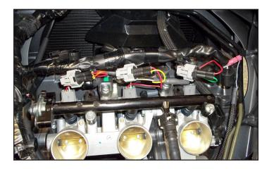
13 Plug the PC6 wiring harness in-line of each Fuel Injector and the stock wiring harness.
