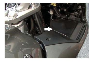
4 Remove the battery cover from the right side of the bike to access the bike's battery.
