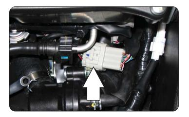
6 Unplug the connector from the throttle bodies to the main wiring harness as shown.
