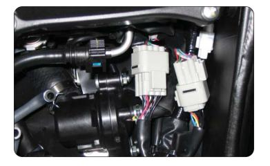
7 Attach the connectors from the PC6 wiring harness to the stock connector as shown.
