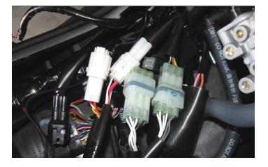
6 Plug the connectors from the PC6 in-line of the stock wiring harness.
