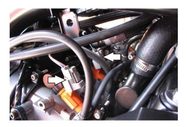
5 Unplug the stock wiring harness from each of the 4 fuel injectors.
