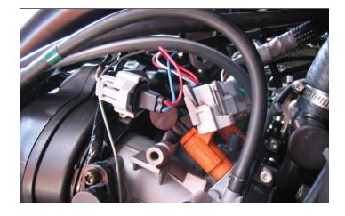
6 Plug the PC6 wiring harness in-line of the stock harness and the fuel injectors.
