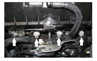
6 Unplug the stock wiring harness from each of the LOWER injectors.
