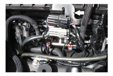
5 Slide the bracket on the back of the air box up to gain access to the injector connectors.
