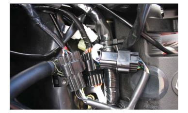
7 Attach the connectors from the PC6 to the stock connector as shown.
