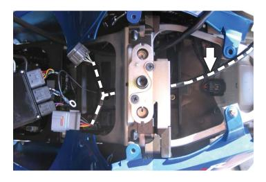
4 Slide the junction box that is under the main seat from it's rubber sleeve.
