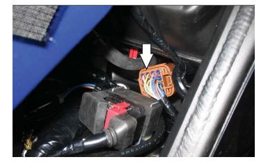
6 Unplug the BROWN 16-pin connector from the throttle bodies as shown.
