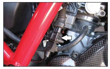
15 Unplug the crank position sensor connector on the right side of the motorcycle.
