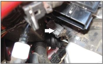
13 Unplug the stock wiring harness from the front injector.
