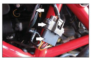
12 Plug the PC6 connectors in-line of the stock wiring harness and Throttle Position Sensor.
