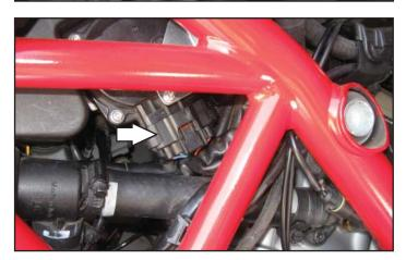
10 Unplug the stock wiring harness from the rear injector.
