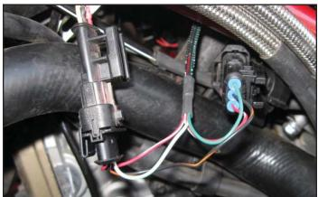
9 Unplug the stock wiring harness from the Throttle Position Sensor (TPS).
