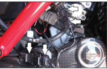
16 Plug the PC6 connectors in-line of the crank position sensor and wiring harness.
