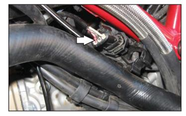
8 Plug the pair of PC6 connectors with the GREEN wires in-line of the stock ignition coil and wiring harness.
