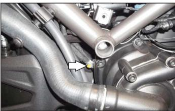
12 Use the remaining Positap to attach the single unterminated GREY/WHITE wire of the PC6 to the stock GREEN/WHITE wire of the bike's Engine Temperature Sensor connector.
