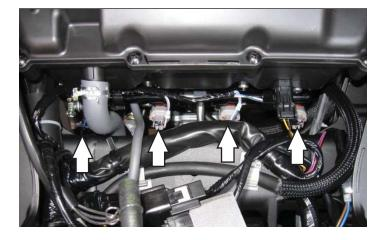
6 Unplug the stock wiring harness from each of the 4 injectors.
