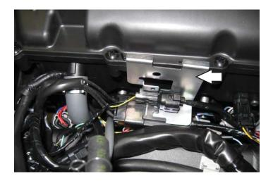
5 Slide the bracket at the rear of the air box upwards.
