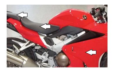
1 Remove the seats, the plastic panel below the rider's seat that covers the top of the battery, and remove the right and left side mid-fairings.
