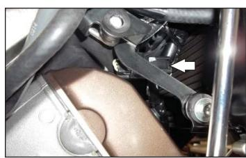
7 Plug the pair of 2-pin PC6 connectors in-line of the stock Crank Position Sensor connectors.
