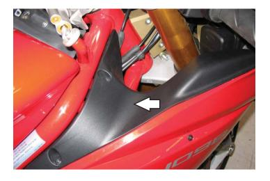
4 Remove the inner fairing cover on the right hand side.
