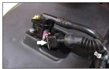
9 Plug the PC6 leads with YELLOW colored wires from the PC6 in-line of the stock wiring harness and rear fuel injector.
