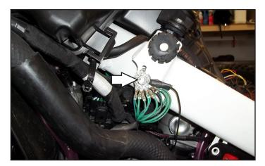
9 Unplug the stock wiring harness from the Crank Position Sensor.
