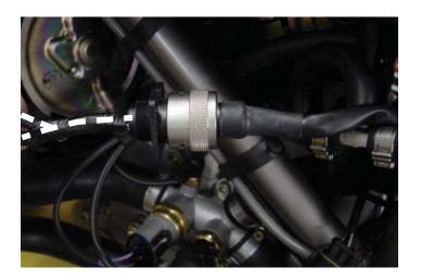
Note: You may want to route the wires for the PC6 from the tail section to this area before plugging it in. This will make for a cleaner installation.
