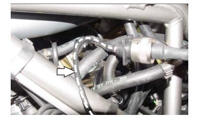
6 Plug the male connector from the PC6 into the stock female connector on the bracket.
