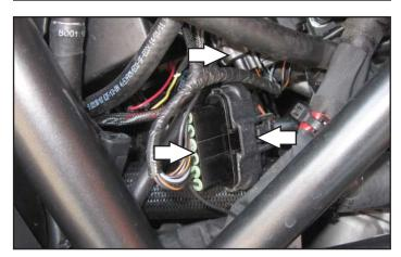
12 Attach the ground wire of the PC6 with the small ring lug to an engine case bolt on the left side.
