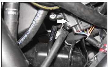
11 Plug the PC6 in-line of the TPS and the stock wiring harness.
