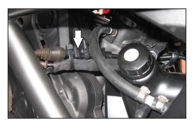
13 Locate and unplug the stock Crank Position Sensor connectors.
