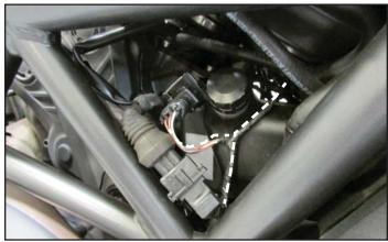
14 Plug the pair of matching PC6 connectors in-line of the stock Crank Position Sensor connectors.
