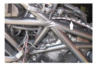
4 Lay the PC6 in the tool kit area under the seat and route the harness going along the left hand side of the frame. Route the harness on the inside of the frame and come out near the rear throttle body.
