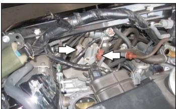
12 Plug the PC6 wiring harness in-line of the fuel injectors and the stock wiring harness.
