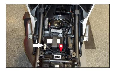
Attach the ground wire of the PC6 to the negative (-) side of the battery.
