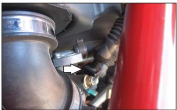
9 Plug the pair of PC6 leads with ORANGE colored wires in-line of the front fuel injector and the stock wiring harness.
