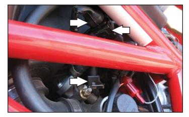
8 Unplug the stock wiring harness from the front fuel injector.
