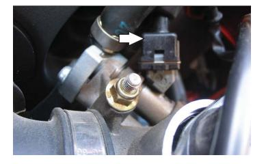
Unplug the stock wiring harness from the rear fuel injector.
