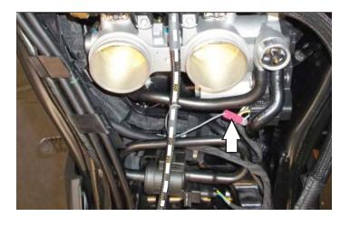
8 Using the supplied posi-tap, attach the GREY wire from the PC6 wiring harness to the stock LIGHT BLUE wire (pin position #2) of the bike's Throttle Body Servo connector.
