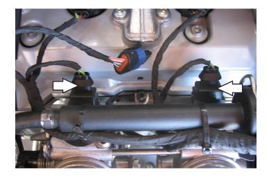
2 Unplug the stock wiring harness from both fuel injectors.
