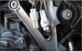
11 Plug the WHITE 2-pin connectors from the PC6 wiring harness in-line of the stock Crank Position Sensor connectors.
