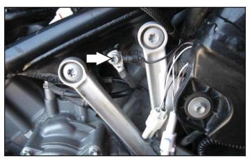
12 Secure the PC6 ground wire with the small ring lug to the stock common ground location on the right side of the frame.
