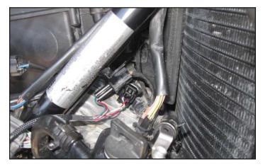
15 Unplug the stock wiring harness from the Rear Ignition Coil.
