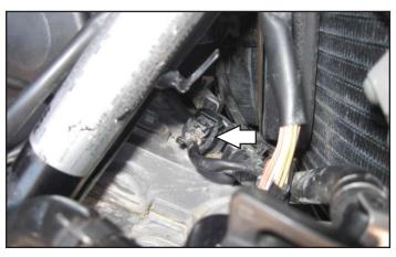
13 Unplug the stock wiring harness from the Front Ignition Coil.
