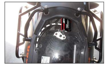
7 Route the PC6 wiring harness inside of the frame rails and go towards the front of the engine.
