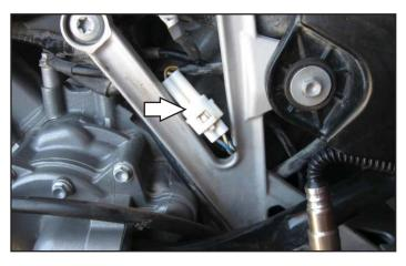
10 Locate the stock Crank Position Sensor connectors on the right side of the motorcycle. Unplug this connection.
