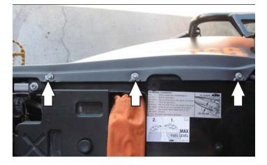
4 Remove the three bolts for the tail section on the right hand side.
