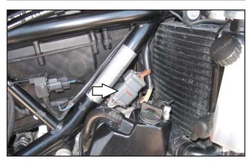
9 Plug the PC6 main connectors in-line of the stock wiring harness.
