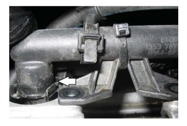
There are two ways to access the fuel injectors. Either remove the entire throttle bodies from the intake manifolds (recommended to replace hose clamps) or follow these instructions.
