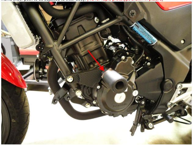
9. With bodywork mounted, install right frame slider puck using 10 X 1.25 X 80 (99-HB-SH10125080) socket cap bolt. Use one drop of blue thread locker on puck bolt and adjust the left frame slider puck to clear bodywork and torque down 30 to 32ft lbs. Red arrow illustrates the flat side of frame slider puck to be adjusted to clear body. (NOTE: Rapid prototype shown in picture)
