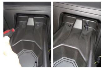
5. Remove push rivets (x2). THEN GO TO STEP 15.
