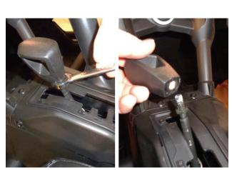
2. Securely chock vehicle's wheels, then loosen jam nut and remove shift knob.
