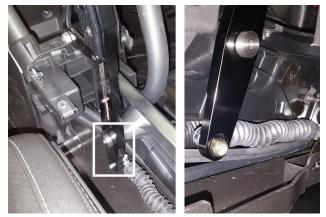
Install shifter stick by inserting spacer through pivot bore then secure shifter cable by tightening nut (removed step 19).
