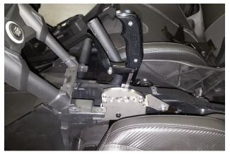
Now that shifter components have been assembled, go back and completely tighten fasteners from the previous steps in this order: Steps 33, 34, 35, 32.
