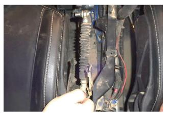
26. Lift cable support out of frame.
