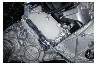
If necessary, adjust shifter cable nut for precision and alignment with transmission as you shift through each gear.
