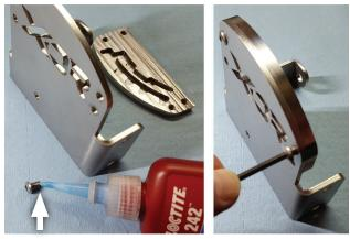
Apply loctite to screws (x4) and use them to fasten gate mount (2) to gate plate (4).
