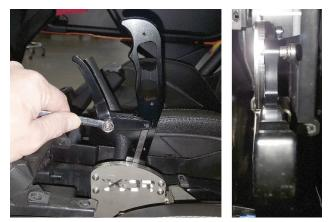
40. Remove and retain lock nut, shoulder bolt, spring washer and shift lever from shifter stick.
