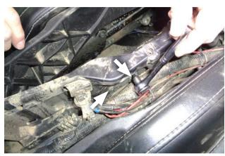
25. Remove screws (x2) securing right side of cable support.
