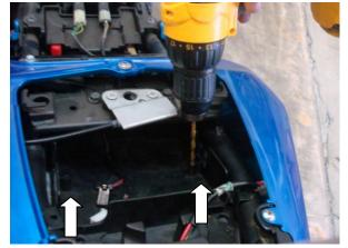
7. Drill out pop rivets though storage compartment, this will hold the pieces together, and will be the mounting location for your license plate.
