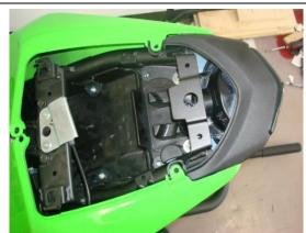
9. Hold all stock pieces together once properly aligned install mounting bolts. Please note that this may require assistance in lining up holes of stock tail section due to snug fit.
