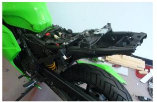
1. Remove seats and proceed to undo mounting bolts for the tail section. Also remove passenger foot pegs. Disconnect signal light and license plate light wires to remove tail light and mud flap completely
