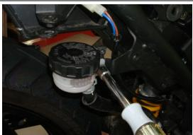
2. Remove bolt holding rear brake reservoir, and move reservoir out of way for installation. Make sure brake reservoir is upright to prevent any leaks. Also place cloth over reservoir bracket to prevent from scratching undertail during installation.
