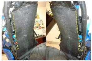
5. More photos of the trimming. Once you have trimmed the glove box. Install new undertail by lining up with trimmed battery box. Make sure everything is in place and holes are mounted up. Slide tail light into undertail.
