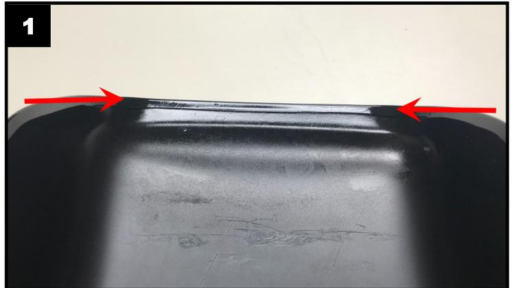
4. Test fit the new Integrated LED Taillight to underside folded lip of the fender. Make sure it is centered, then mark the position with a grease pencil for a guide. **NOTE:** the Integrated LED Taillight mounts on the folded lip of the fender not behind it.
