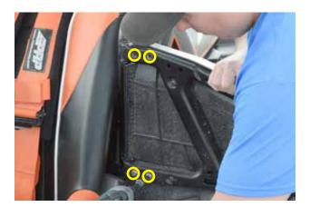
2. Remove Stock Door Using a T40 Torx, remove the 4 hinge bolts (2 top and 2 bottom) from the stock door.
