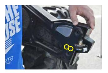
1a. Using your T25 Torx, remove the small bolts holding on the door latch, just behind the latch mechanism.There are 2 per door.
