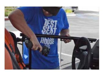
Tighten the T40 bolts on the hinge. Once tight, open and close the door a few times making sure the latch is striking correctly and closing completely.
