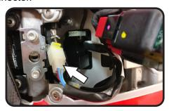
While securely supporting the stock fender assembly, remove the three bolts securing the fender assembly to the frame from below. Carefully remove the stock fender assembly making sure not to damage the connectors in the process.
