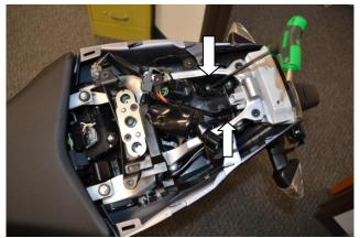
3a) Unbolt the 25mm allen bolts located on the inside of your glove box holding on your stock mudflap. See close up picture on 3b for reference.
