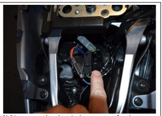
2) Disconnect the electrical connectors for the turn signals, license plate light, and tail light.
