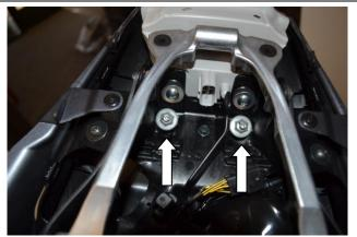
6b) Secure tag using the 2 stock 5mm allen bolts & the 2 locking washers provided. \*Note bolts will bolt from the bottom upwards. DO NOT OVERTIGHTEN!
