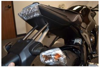
4) Gently remove the stock mud-flap assembly by pulling it out. Be careful feeding wires through the holes in the stock pieces.
