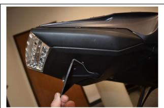
6a) Now that your Tag Bracket is ready for installation, feed the new wires through the existing holes for the plate light wires and insert front tip first then lift up into place.
