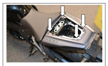
1) Remove stock passenger seat and remove the 4 4mm allen bolts holding tail section on. Slide tail section backwards and up to remove.
