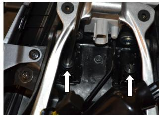
3b) Remove these two bolts and the brackets that they are holding on.
