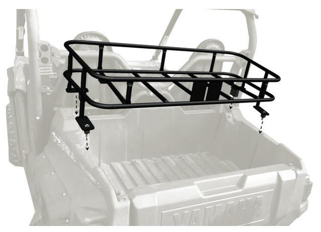
Install the Cargo Rack by locating the rubber feet into the slots of the bed as shown
