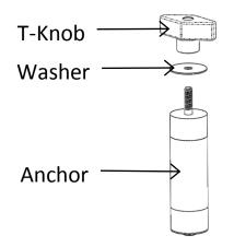
Remove the T-Knob and Washer from each of the Anchor Assemblies.
