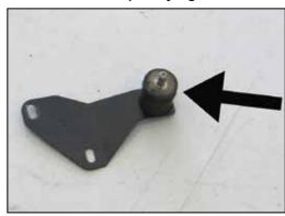
21. Install the long rubber mounted stud to the heat shield mounting bracket (083118) as shown and secure with the provided hardware.
