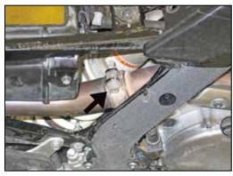
5. Loosen the clamp which secures the muffler inlet to the exhaust pipe.
