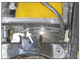
9. Loosen the hose clamp which secures the intake hose to the air box.
