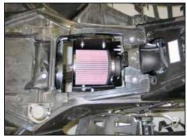
27. Tighten the hose clamps that secure the intake tube to the throttle body and air filter. Align the heat shield and tighten all of the mounting hardware.
