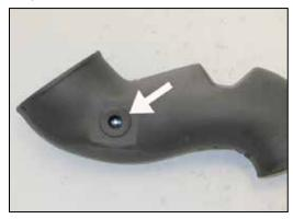
14. Install the provided grommet into the intake tube as shown.
