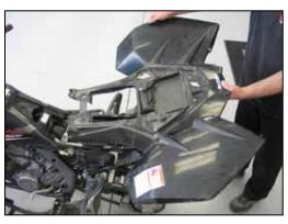
4. Remove the rear body work from the vehicle.
