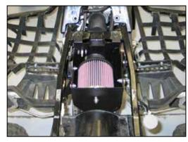
24. Install the heat shield and filter assembly into the frame from the bottom. Install the intake tube into the filter; install the rubber mounted studs into the air box mounting holes located in the frame tabs. Once the assembly is installed, secure the rubber mounted studs to the chassis with the provided hardware.
