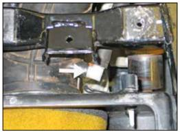
8. Disconnect the crank case vent hose from the air box.
