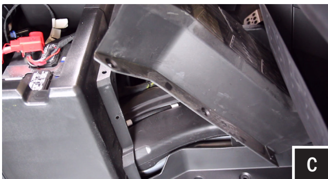
C. Using a panel removal tool, extract the (8) push pins to remove the center driveline center column cover.
