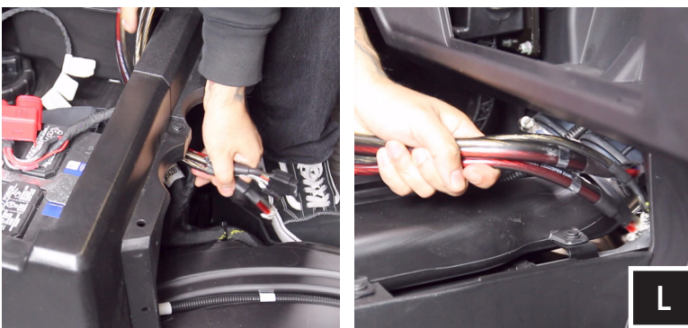
L. Pull all cables and wiring around battery and through the center of vehicle away from any moving parts and sharp metal. Connect to the amplifier.
