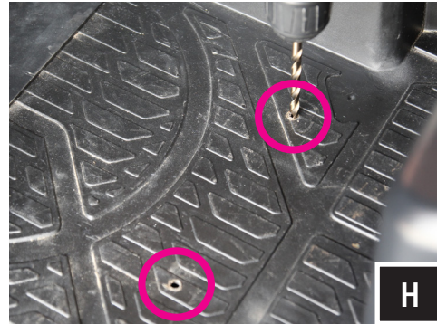
H. Once marked, remove the enclosure. Using a 13/64" drill bit, drill pilot holes at your marked points. Be sure to penetrate through the chassis lying beneath the floorboard.
