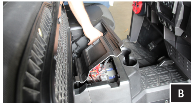
B. Flip up passenger seat and remove center tray to access battery. Disconnect the negative battery cable from the battery.
