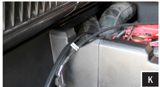
K. Pull the harness into the battery cavity.
