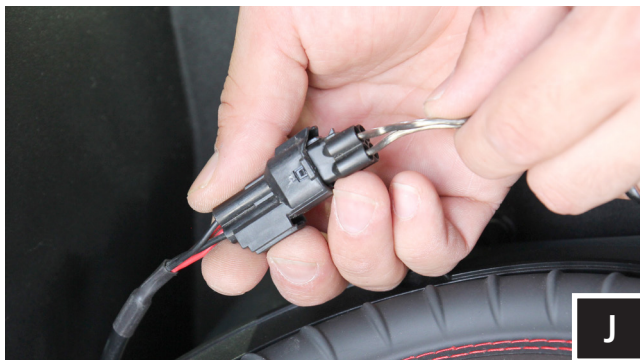
J. Connect sub to harness B-H1151
