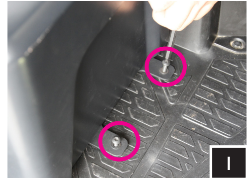
I. Re-install the sub-enclosure. Secure the front mounting tabs with the kit provide T30 torx self-tapping screws.
