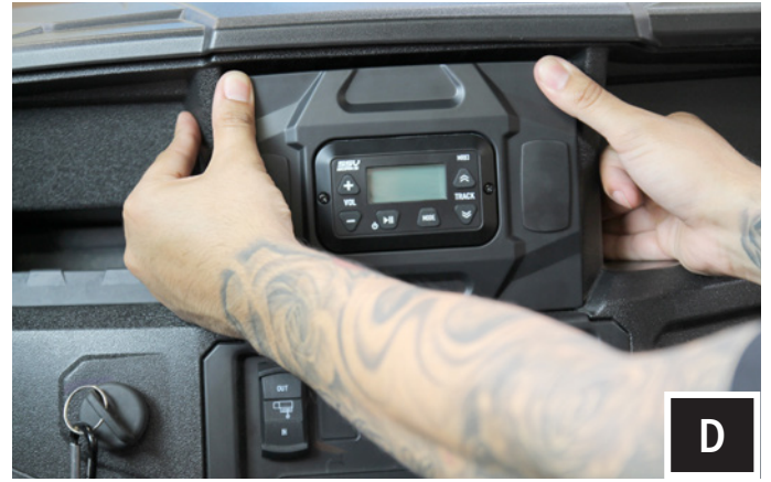
D. With both thumbs press the top corners until the kit snaps into place.
