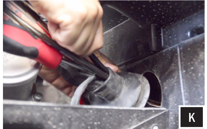
K. Unwrap the tape from rubber grommet and feed the power/ground wire for the Amp through the grommet as well as the rear speaker harness H1151 (rear speaker harness to be used for rear speaker expansion pods).
