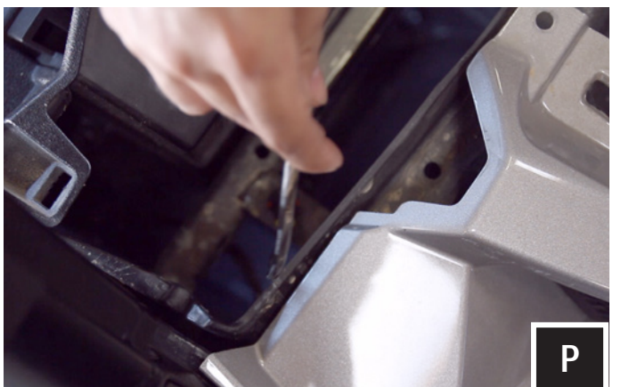
P. Feed each side of the H1149 harness down through the open cavity on top of the dash towards the driver and passenger footwell.
