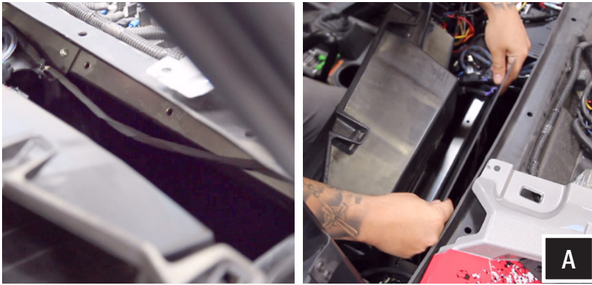
A. For this step you will need the sub enclosure mounting plate as well as two (2) M5 screws, two (2) 8mm nuts and four (4) M5 washers. Place the mounting plate on the factory dash cross member bar behind the glovebox. Match up the holes from the plate and the bar to insert the M5 screws and washers from top. Use the 8mm nuts and washers to fasten from underneath.
