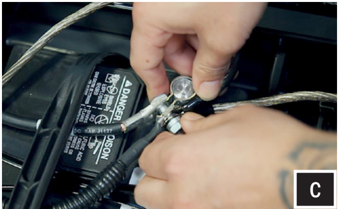
C. (If you have decided to disconnect the negative terminal as suggested earlier). Reconnect the negative battery cable. Remove the nut and connect the two ground cables. Reinstall nut and tighten.
