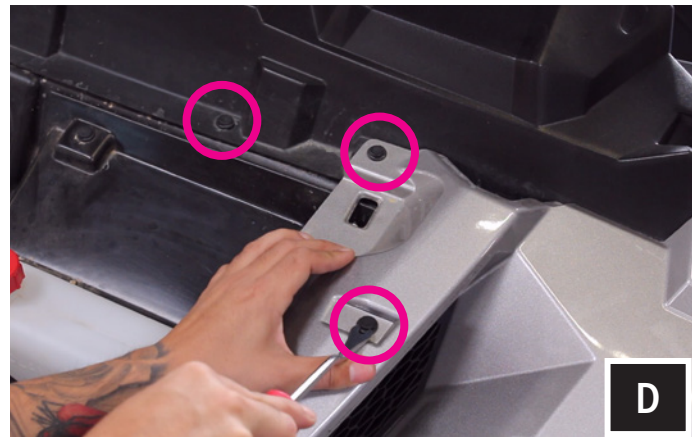
D. Start to remove dash by removing the six (6) push pins under the hood.
