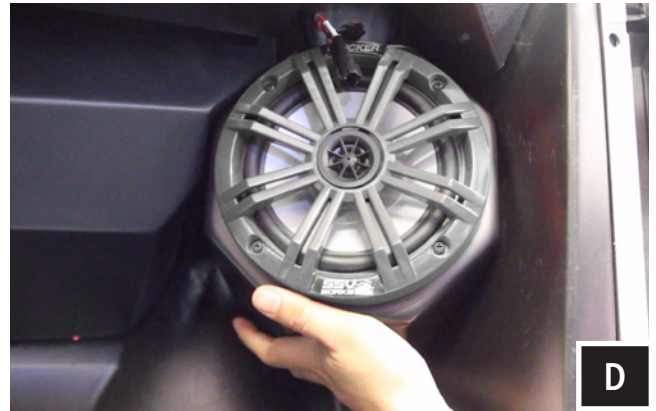
D. Place enclosure in location for mounting.
