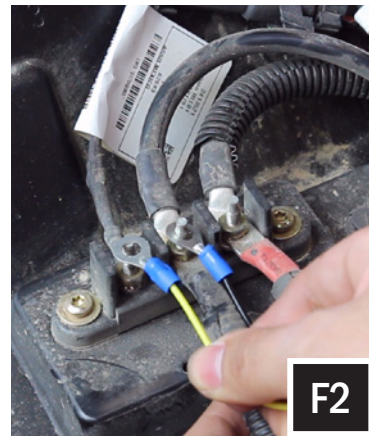
F. At the Bus Bar terminal located under the hood, unscrew the nut on the second position terminal and attach the black Ground wire. Refasten the nut. Then connect the yellow Power wire to either the constant terminal (F1) or the accessory terminal (F2). Refasten the nut.
