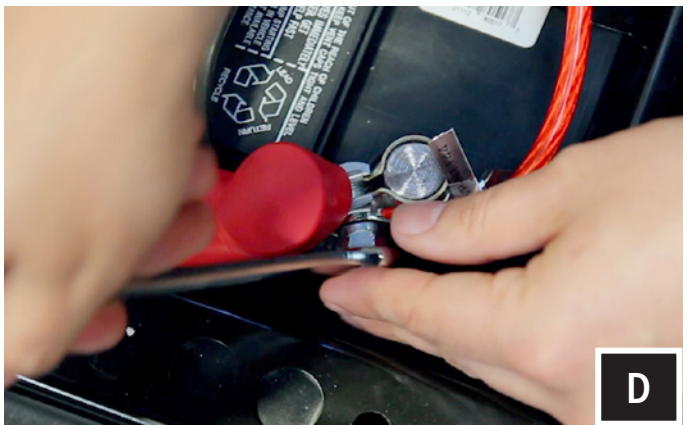
D. Unscrew the factory nut on the positive battery terminal. Install the 2 power cables to the screw on the positive battery terminal. Re-install the factory nut.
