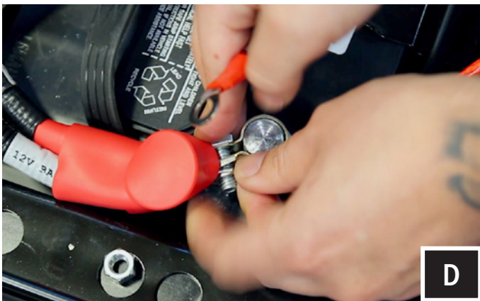
D. Unscrew the factory nut on the positive battery terminal. Install the 2 power cables to the screw on the positive battery terminal. Re-install the factory nut.
