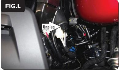
18 Locate and unplug the stock Crank Position Sensor connectors (Fig. L).
