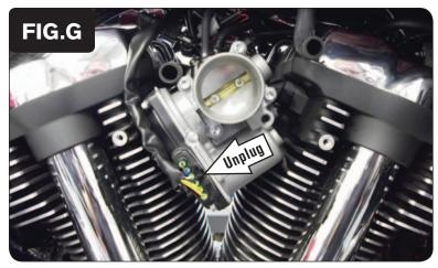
13 Unplug the throttle body servo connector from the throttle body (Fig. G).
