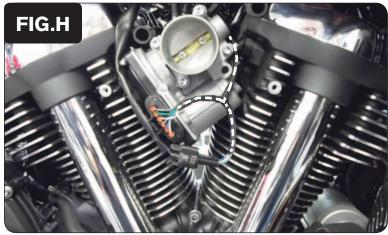
14 Plug the PCV wiring harness in-line of the throttle body and the stock wiring harness (Fig. H).
