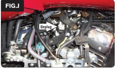
From the left side of the engine, locate and unplug the rear cylinder fuel injector (Fig. J).
