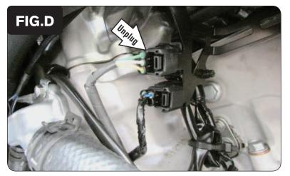
9 Unplug the stock Gear Position Sensor connectors (Fig. D).
