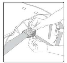
After placing the soft top over your stock roll cage, secure the self-fastening straps from underneath to the roll bar.
