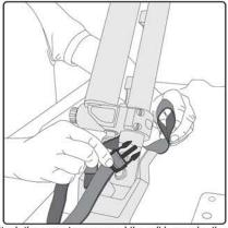
Attach the rear straps around the roll bar under the shock by passing the strap through the webbing loop and pull tight. Connect to the female buckle on the soft roof and pull snug but not tight.
