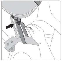
Attach the side straps around the roll bar under the seat belt bolts by passing the strap through the webbing loop and pull tight. Connect to the female buckle on the soft roof and pull snug but not tight.
