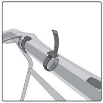
Once rolled tightly and under the roll bar, pass the self-fastening straps around the roll bar and then around the tightly rolled panel. Insert the strap thru the loop on the top of the cover, then attach to itself.
