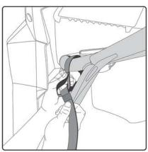
To secure the front, remove the male buckle from one of the straps with a loop and pass around the roll bar located above front wheels under the vehicle.
