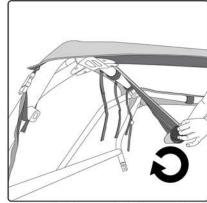
When opening the sunroof. Unzip and roll back as shown. It is important for the roll to go towards the back under the zippered panel.
