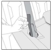
Once secure on the roll bar, feed the end up through the hole where the roll bar meets the side of the hood plastics. Connect to the female buckle on the soft roof and pull snug but not tight.
