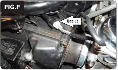
Locate and unplug the stock wiring harness for the bike's Crank Position Sensor (Fig. F).
