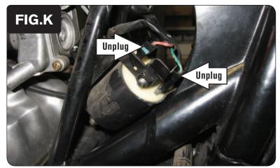
17 Unplug both of the stock wires from the ignition coil (Fig. K).
