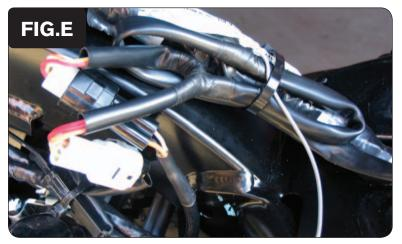
Using the supplied zip tie, secure the PCV harness to the main wiring harness (Fig. E).
