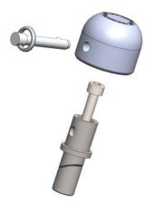
A note for racers: If your tech inspector wants you to safety wire these (most will not) then you simply need to orient the pins so that the pull on the pin is both clockwise and down (so that it acts to both tighten the bolt and pull the pin into the puck)
