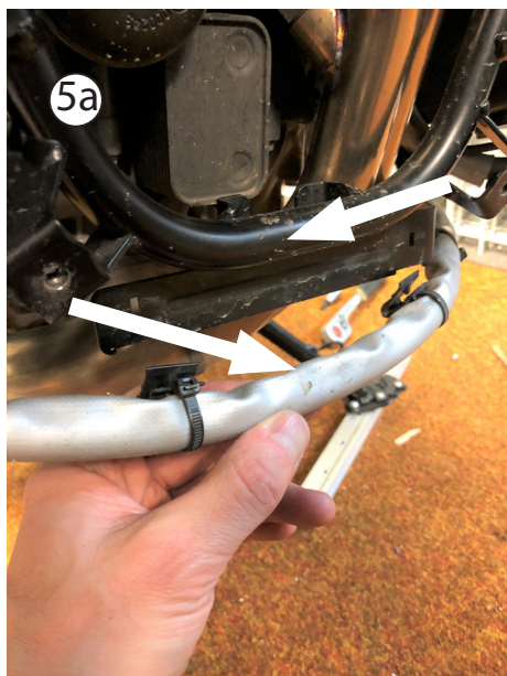
⑤a Carefully unclip the fuel line from the skid plate sub-frame. Remove the skid plate sub-frame. ⑤b
