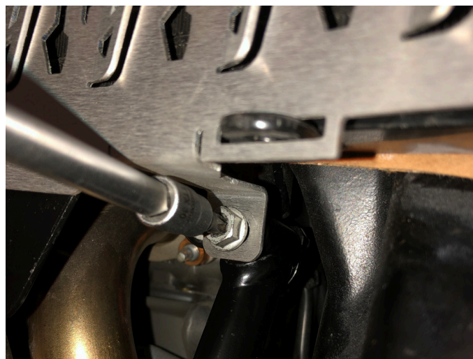
⑦ Position the sub-frame mounting boss behind the radiator guard mounting tab and insert the screw through both and thread it into the frame hand tight. PRO TIP: Press the radiator guard mounting tab towards the back of the bike to make it easier to thread the screw. Repeat for the other side. Tighten both screws to 18 NM. Tighten the top screws to 12 NM.
