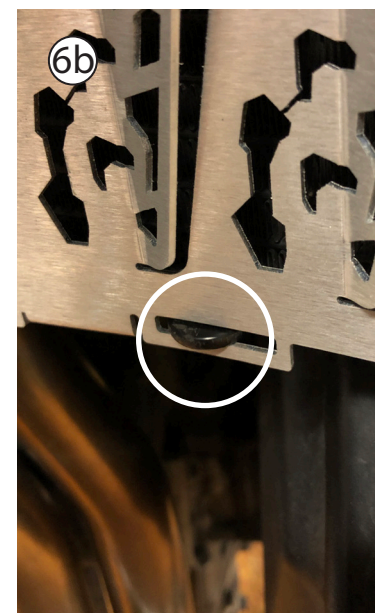
⑥a Position the radiator guard so that the top tabs align with the mounting holes and so that the bottom radiator tabs fit through the slots on the bottom of the radiator guard as shown. Install the top screws loosely securing the radiator guard. ⑥b
