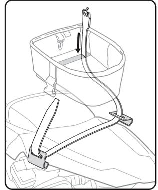
Thread Pronghorn Strap, small end down, through the slot on the bottom of Klamath. Slide on two fender hooks, facing each other as shown. Position Klamath as desired, secure hooks on either side of fender. Repeat for second strap.
