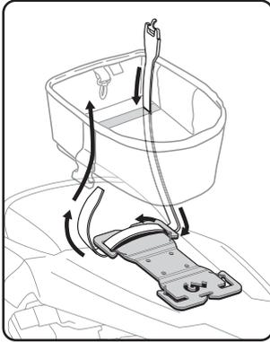
For best compatibility with Klamath, position GL Tail Rack lengthwise. Thread Pronghorn Strap, small end down, through the slot on the bottom of Klamath. Pass the strap through the carabiner clip slots on the tail rack, then back through the opposite slot on Klamath. Repeat for second strap.
