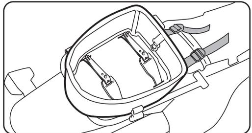
Remove webbing straps if not needed, or use them to apply forward tension on fender hooks. Re-attach lid and insert included divider and waterproof Dry Pod.
